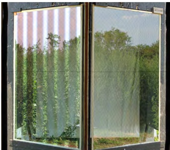
Bird's-eye view in the test tunnel. Pilkington AviSafe™ exterior view: highly effective as protection against bird collision, barely visible from the interior (left: test pane, right: reference pane).
