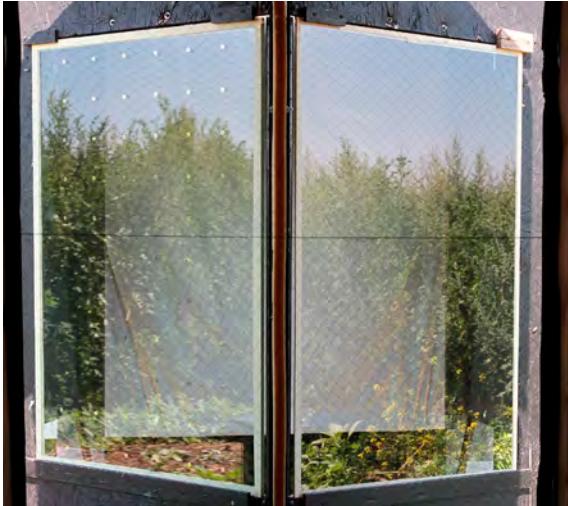
Eastman Saflex® FlySafe™ SEEN shiny 9/90: metallic dots, 9 mm in diameter and 90 mm apart: highly effective and – due to high reflectance – also suitable for surface 2 (left: test pane, right: reference pane).
