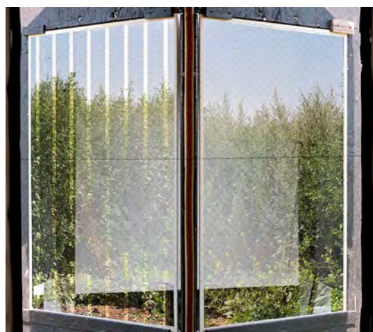
A marking currently being developed by the Fraunhofer Institute for Solar Energy Systems (ISE), with transparent stripes on surface 1, proved to be highly effective (left: test pane, right: reference pane).
